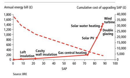
**Figure 2.4:** The cost of improving the SAP rating and the resulting impact on the household energy bill for a typical cavity-walled, detached property on the gas grid (average prices 2003-2005)
