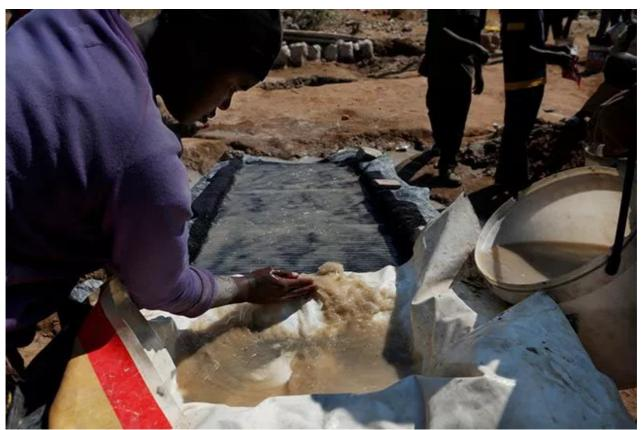
A man-made drainage system where water is used to separate gold from sand. What remains on the carpet are gold particles encroached in impurities. Gold is said to be denser than water and sand particles and would not be washed away by the water as it goes down
