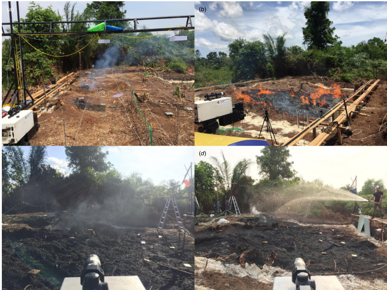
Fig. 5. Photographs showing a typical set-up of OP-FTIR measuring emissions from ember ignition (a, EI4), slash-and-burn (b, SB1), smouldering spread (c, SS23), and water spray suppression (d, SP3).
