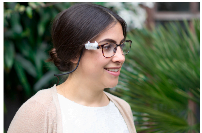
Fig. 1. Multi-device A researcher modeling the Subcam. The camera weighs only 7 g and can be mounted on a pair of research glasses or the participant's own (here); it has about 3 h of autonomy with the internal, and several days with an external battery.
